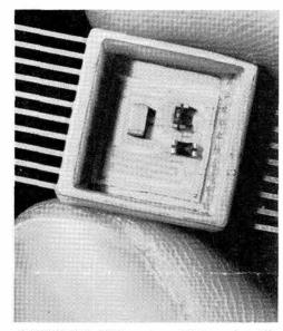
FINGERNAIL SIZE, microminiature hybrid integrated circuit contains a transistor and two capacitors (darker components) interconnected to thin-film resistor and conductor pattern.
